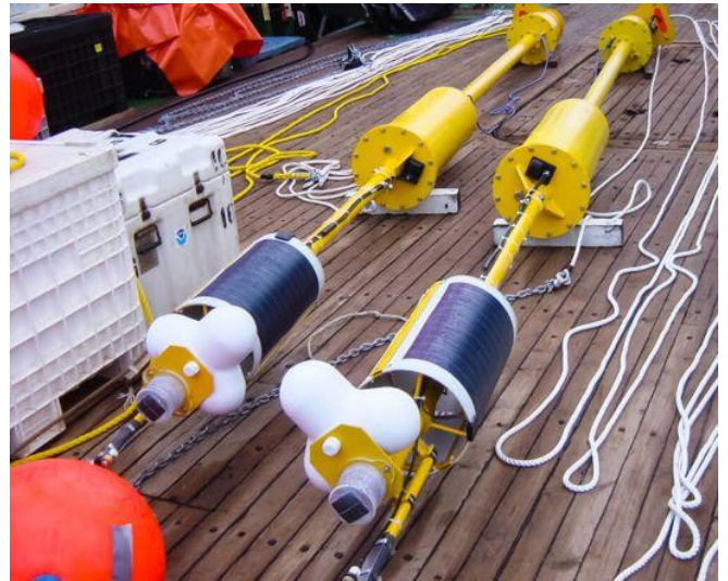
Figure 9: Acoustic monitoring devices that record various marine species including whale songs and dolphin clicks.
